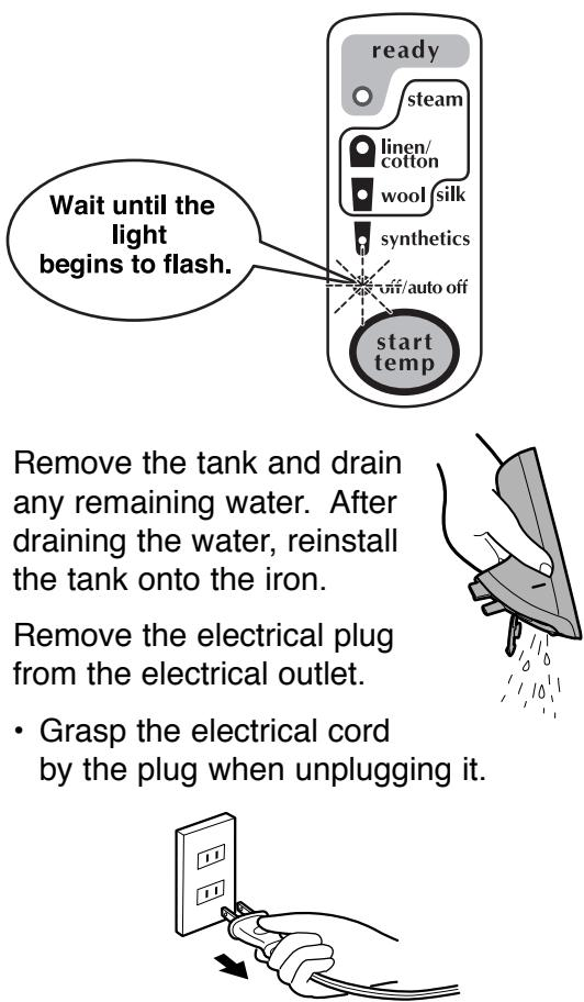
3. Remove the tank and drain any remaining water. After draining the water, reinstall the tank onto the iron.
